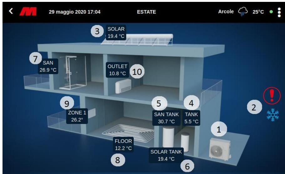
The image above shows the image with all configurations enabled. The configurations are enabled by configuring the corresponding probes on the heat pump.
