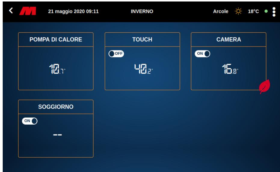
In this page are displayed the configured zones in the control unit and the heat pump. On the first rectangle there is the discharge probe e the eventual alarm status.
