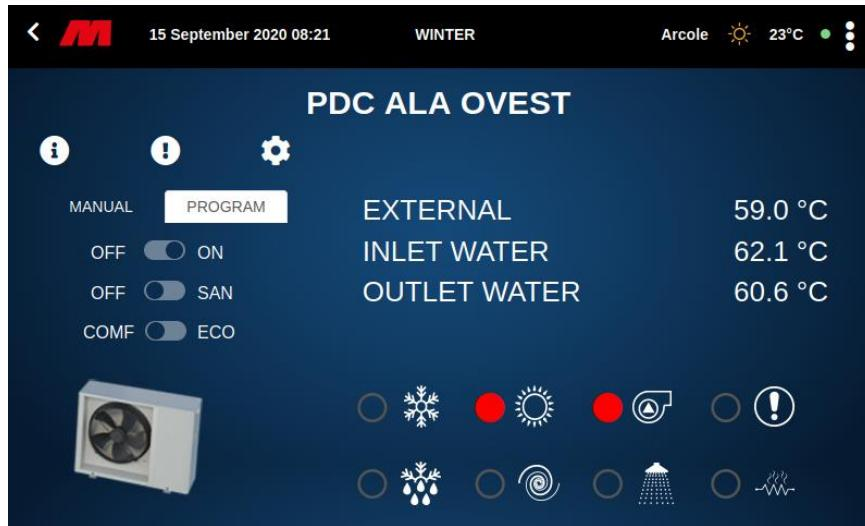
Pressing above the pump image it is possible to access on the screen where the first heat pump is displayed, with the possibility to scroll to the following ones. The PDCs are sorted by Modbus ID and the first one has the minor ID.
